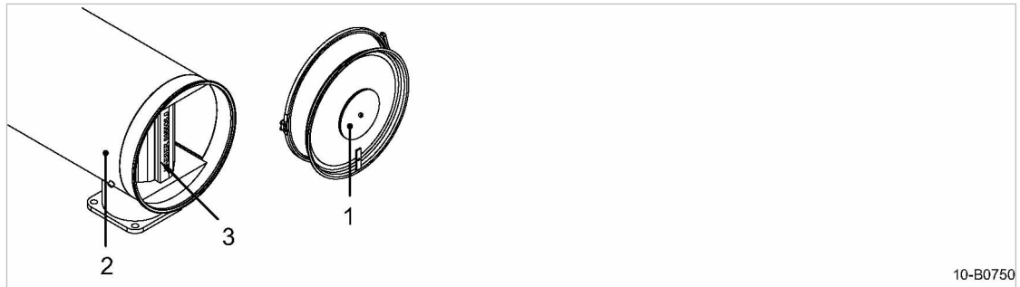
Fig. 32 Changing the air filter
