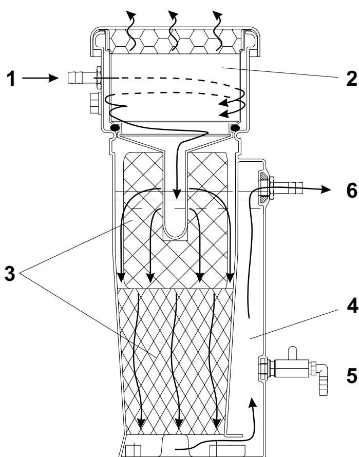
The oil-contaminated condensate can be fed under pressure to the KCF unit (1).
