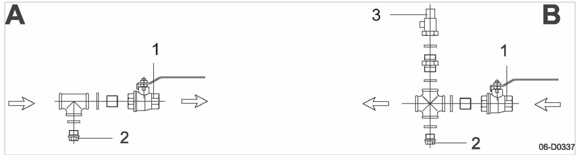
Fig. 25 Connecting the water cooling
