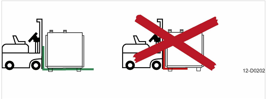
Fig. 32 Transporting with a forklift truck
