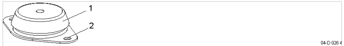
Fig. 21 Machine Mountings ① Machine mounting ② Holes for anchor bolts to fix the mounting to the floor.
