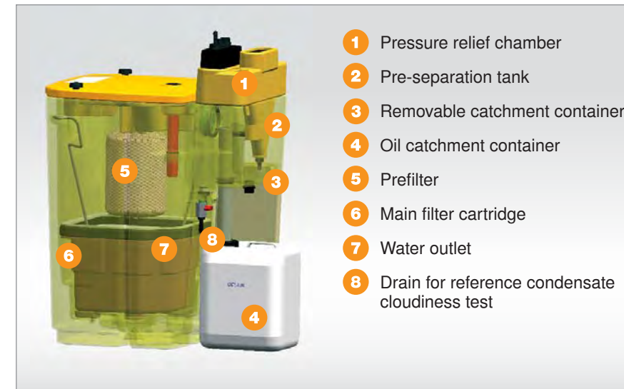
Fig. 2: Condensate separation system for compressed air technology using the gravity principle (functional diagram)
