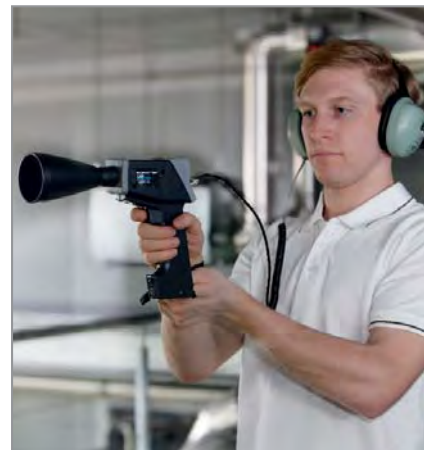
Fig. 4: Leakage location using ultrasound
