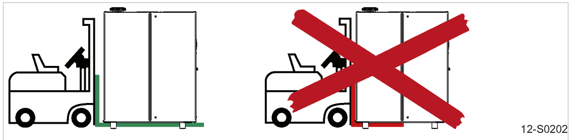
Fig. 34 Transporting with a forklift truck
