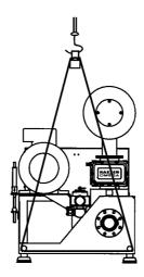
No side forces should act upon the package when transporting with a sling. Always use a spreader!
