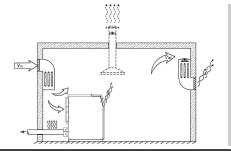
It is recommended to extract the exhaust air from the upper third of the room as this is where the heat collects. The room ventilation openings should be arranged that the current of cooling air flowing through the room passes over the blower inlet and exhaust ports and, if possible, should leave no stagnant air in the room. (A thermal short circuit must be avoided, i.e. discharged cooling air must not find its way to the cooling air inlet.)
