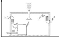
It is recommended to extract the exhaust air from the upper third of the room as this is where the heat collects. The room ventilation openings should be arranged that the current of cooling air flowing through the room passes over the blower inlet and exhaust ports and, if possible, should leave no stagnant air in the room. (A thermal short circuit must be avoided, i.e. discharged cooling air must not find its way to the cooling air inlet.)
