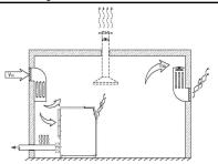
It is recommended to extract the exhaust air from the upper third of the room as this is where the heat collects. The room ventilation openings should be arranged that th current of cooling air flowing through the room passes over the blower inlet and exhaust ports and, if possible, should leave no stagnant air in the room. (A thermal short circuit must be avoided, i.e. discharged cooling air must not find its way to the cooling air inlet.)
