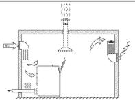
is where the heat collects. The room ventilation openings should be arranged that the current of cooling air flowing through the room passes over the blower inlet and exhaust ports and, if possible, should leave no stagnant air in the room. (A thermal short circuit must be avoided, i.e. discharged cooling air must not find its way to the
