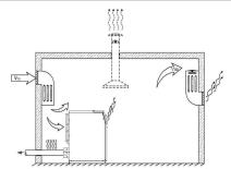
It is recommended to extract the exhaust air from the upper third of the room as this is where the heat collects. The room ventilation openings should be arranged that the current of cooling air flowing through the room passes over the blower inlet and exhaust ports and, if possible, should leave no stagnant air in the room. (A thermal short circuit must be avoided, i.e. discharged cooling air must not find its way to the cooling air inlet.)
