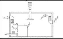
It is recommended to extract the exhaust air from the upper third of the room as this is where the heat collects. The room ventilation openings should be arranged that the current of cooling air flowing through the room passes over the blower inlet and exhaust ports and, if possible, should leave no stagnant air in the room. (A thermal short circuit must be avoided, i.e. discharged cooling air must not find its way to the cooling air inlet.)
