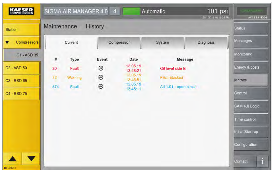
Fig. 134 Menu Maintenance – History – Current for the selected machine
