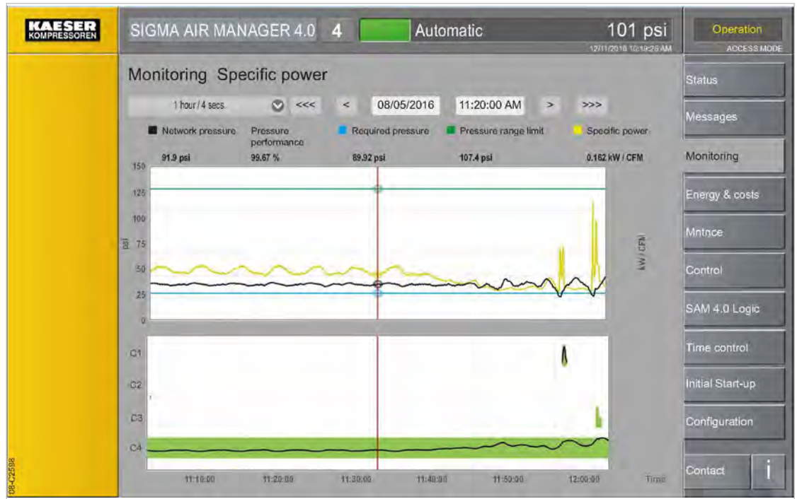
Fig. 112 Menu Monitoring – Specific power
