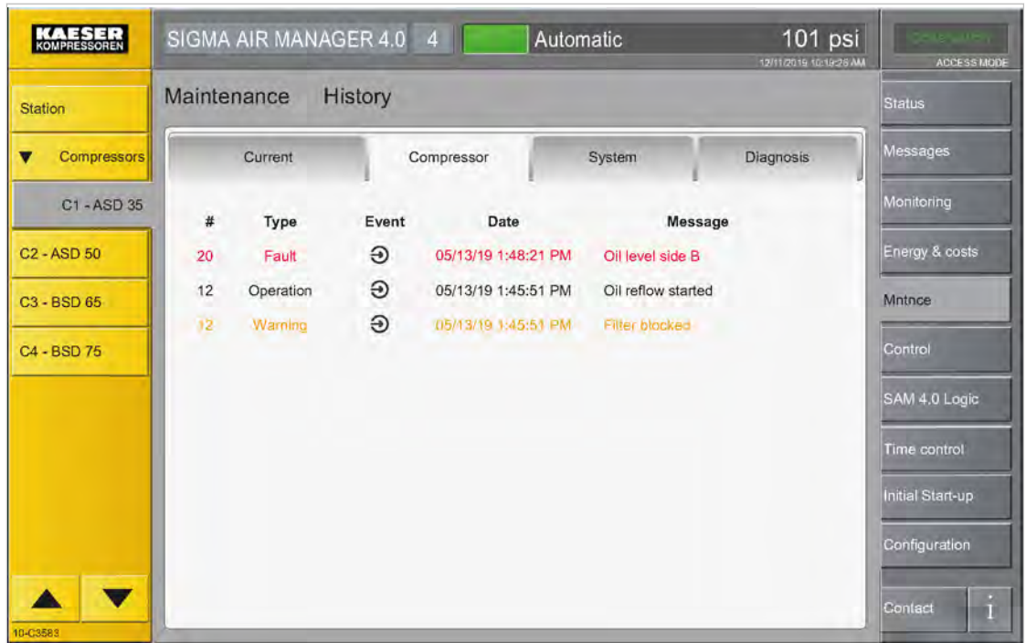
Fig. 135 Menu Maintenance – History – Compressor for the selected machine
