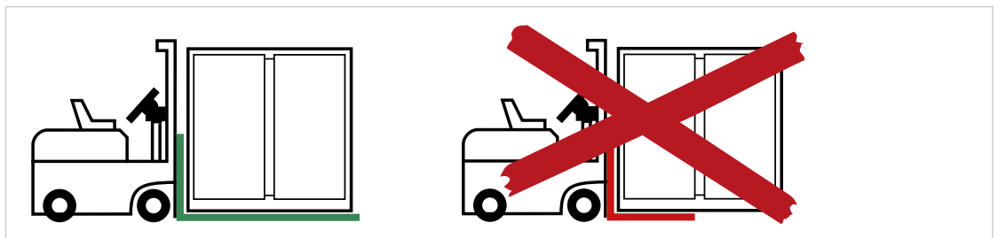
Fig. 20 Transporting by forklift
