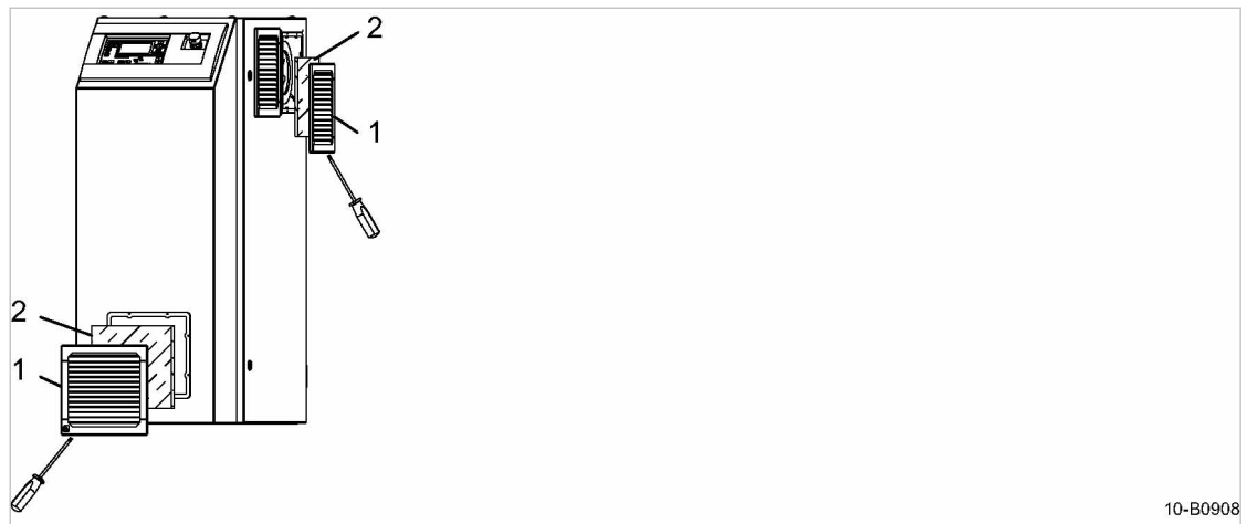
Fig. 24 Control cabinet ventilation grill
