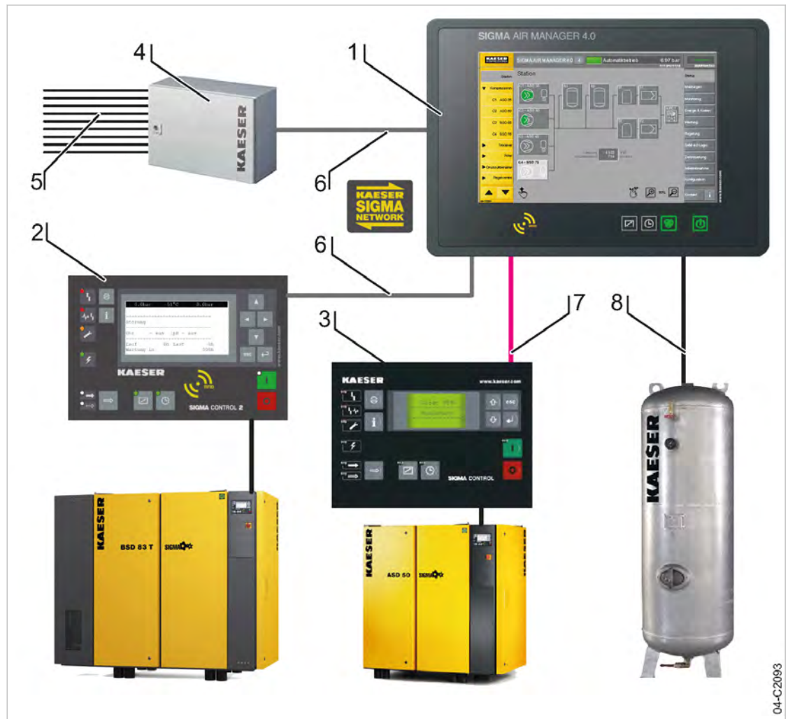
Fig. 2 SIGMA AIR MANAGER 4.0 – Standard design of a compressed air station
