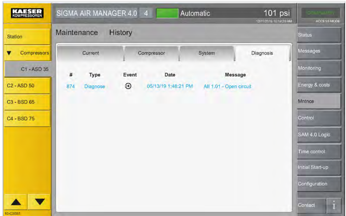
Fig. 137 Menu Maintenance – History – Diagnosis for the selected machine
