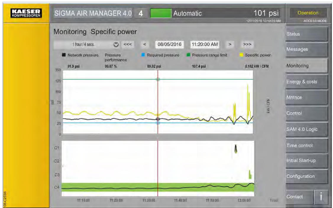
Fig. 112 Menu Monitoring – Specific power
