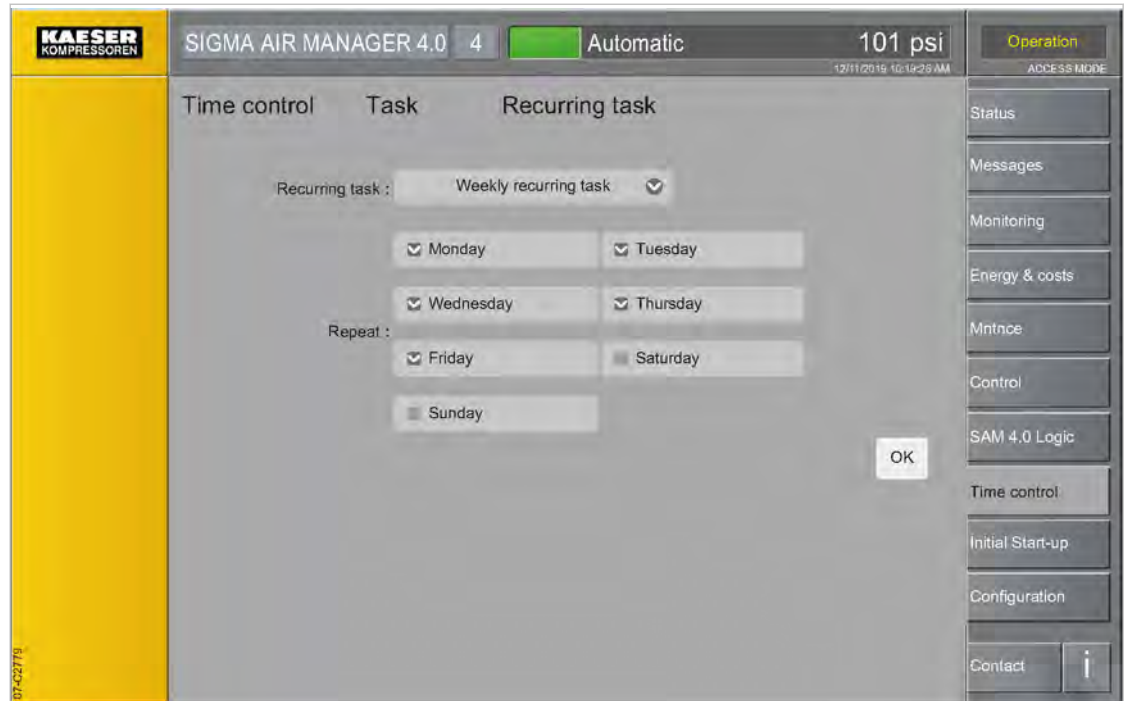
Fig. 77 Menu: Timer control – Task – Recurring task
