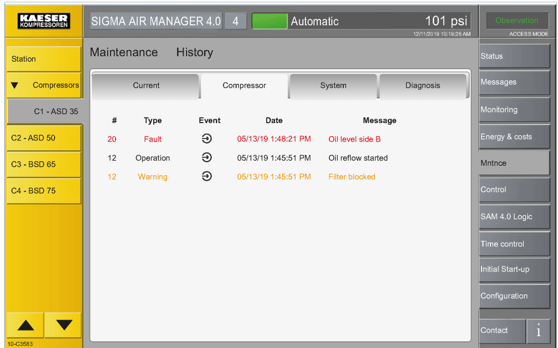
Fig. 136 Menu Maintenance – History – Compressor for the selected machine
