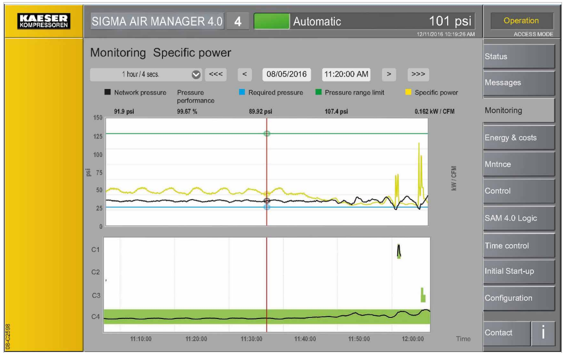
Fig. 113 Menu Monitoring – Specific power
