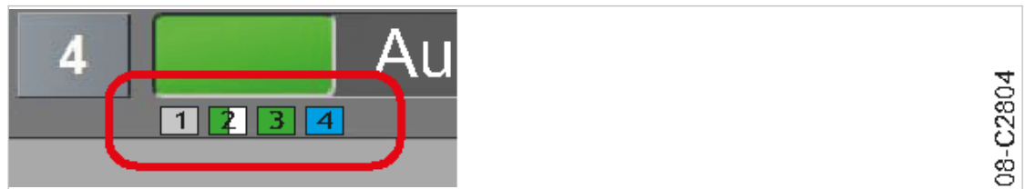
Fig. 52 Status display of the compressed air device in the header
