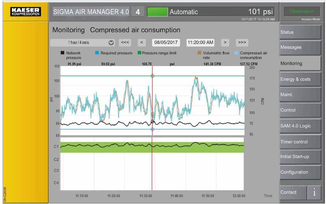
Fig. 112 Menu Monitoring – Compressed air consumption
