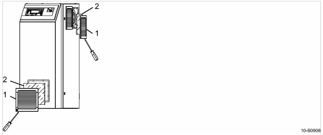
Fig. 24 Control cabinet ventilation
