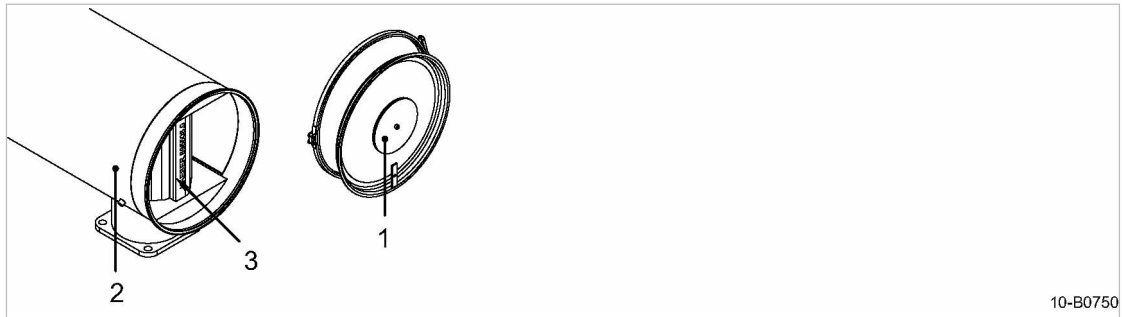
Fig. 30 Changing the air filter
