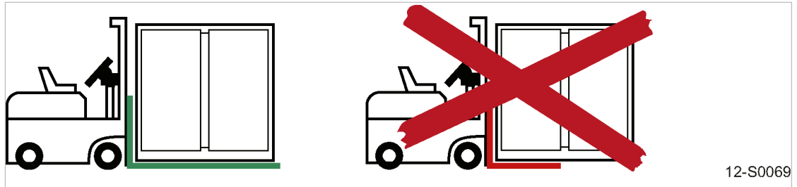
Fig. 52 Transport with a forklift truck
